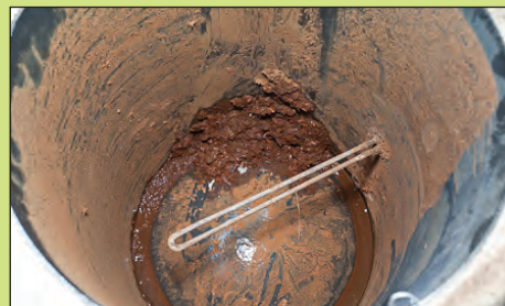
Electric Storage Water Heater After 90 Days Using Unsoftened Water
