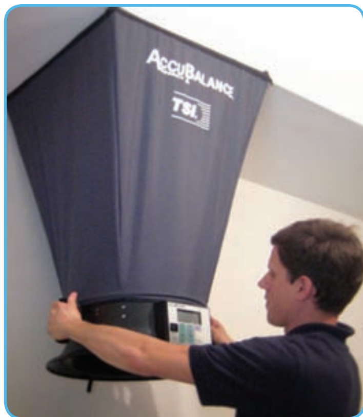
A new requirement: Under ENERGY STAR Version 3.0, a diagnostic test ensures the HVAC system is providing adequate airflow at each room to keep the home comfortable and operating efficiently. photo courtesy of Home Energy Partners
